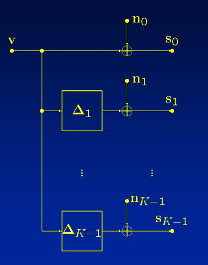
Model for coding with motioncompensated lifted wavelets [Flier! & Girod, 2003]
