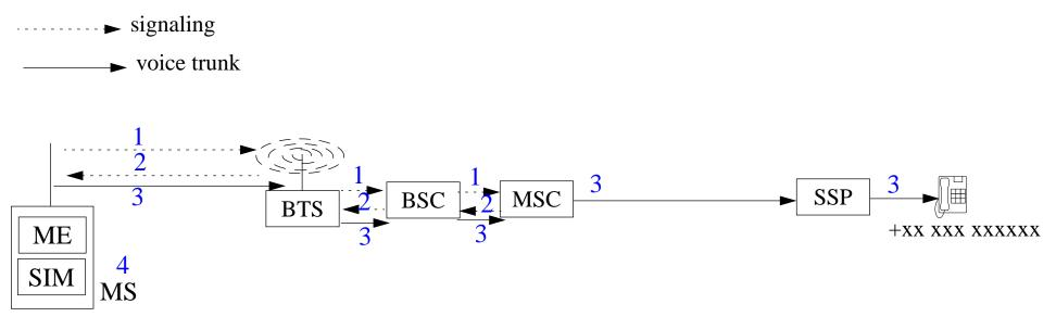
Figure 7: Handset-Based Prepaid call origination
