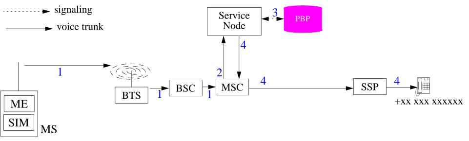
Figure 5: Service Node Prepaid call origination
