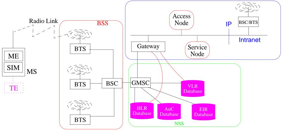
Figure 2: Ericsson's GSM on the Net Architecture
