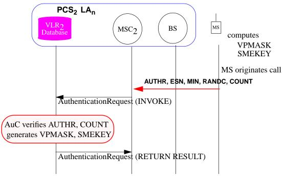
Figure 5: Mobile places a call in PCS<sub>2</sub> using sharing scheme
