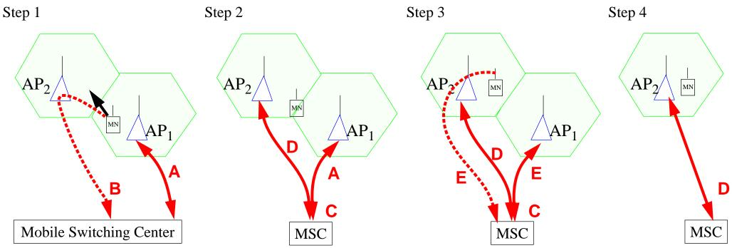
Figure 6: steps in handoff within the control of one MSC (not showing the BSC)
