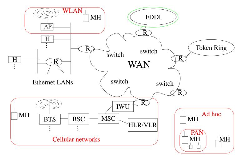
Figure 1: Multiple network technologies - internetworked together
