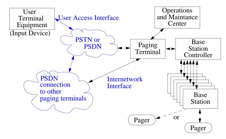
Paging terminal has DB of customers, cap code, pager number, types of msgs, ...; convert voice msg to text (for alphanumeric pagers); store in mailbox for pager; forward to other paging terminals; send to relevant Base Station Controller(s)
