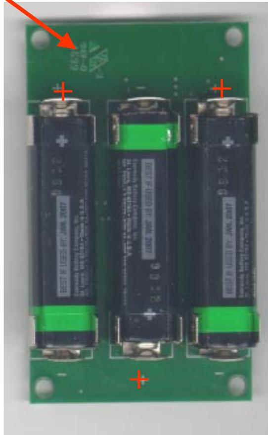
Battery polarity is also silkscreened onto the board.
