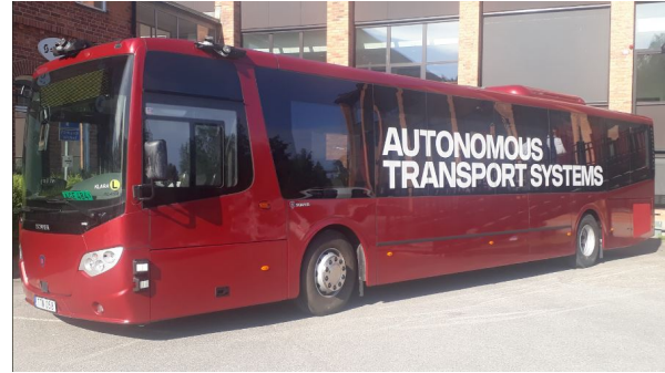
Fig. 1: Autonomous Scania bus equipped with lidar, radar, camera and other sensors.
