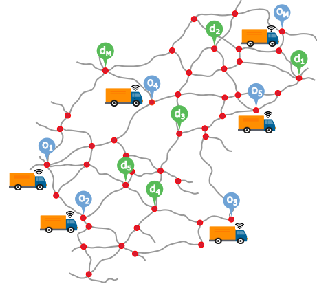
Fig. 1. A graph illustrating the platoon coordination problem considered in this paper, where hubs in the transport network are denoted by red nodes. Origins and destinations are marked by blue and green labels, respectively.
