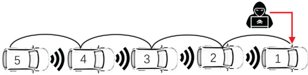
Fig. 1. Platoon of five vehicles, where the position and velocity measurements of vehicle 1 are compromised by a malicious attacker. Each vehicle is able to exchange messages with other vehicles nearby through wireless communication.
