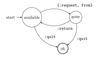
Implement this process in a module Chopstick with a function start/0 that spawns the process and returns the process id. When you spawn the process use spawn\_link/1 to make sure that the chopstick process dies if the mother process dies (and vice verse). This is some skeleton code to give you the structure of the implementation.
