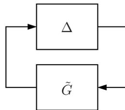
Figure 5.2: A feedback interconnection of  $\tilde{G}$  and  $\Delta$ .
