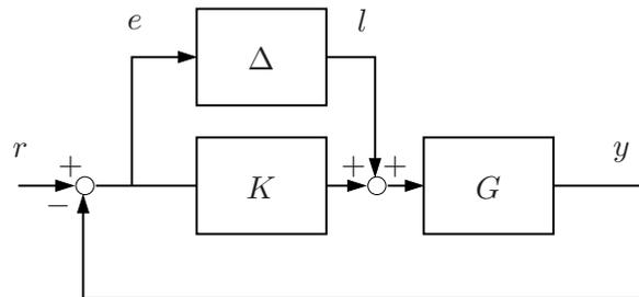
Figure 5.1: A feedback-control system. The plant  $G$  is controlled by the reduced controller  $K_r = K + \Delta$ .
