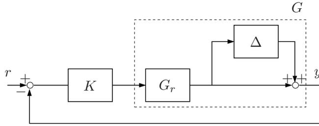
Figure 5.3: A feedback-controlled system. The perturbed reduced plant  $G = (I + \Delta)G_r$  is controlled by the controller  $K$ .
