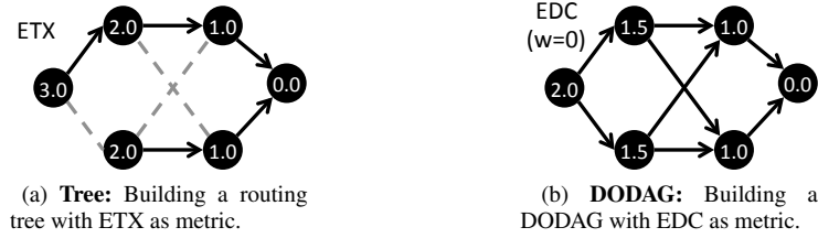
Fig. 7: Topology I: We depict the resulting tree and DODAG when using ETX and EDC, respectively, to build the routing topology. The toy topology highlights that a DODAG build with EDC leads to a dense routing topology when compared to the tree built with ETX. For simplicity, all links are assumed to be reliable, i.e., have a PRR of 1. The values depicted on the nodes represent the routing estimates computed by the respective metrics.
