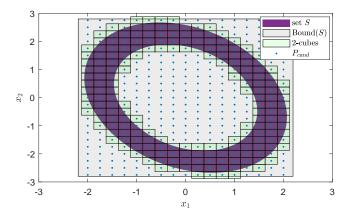
Fig. 1: Grid sampling of a set S in 2-D. Here the set Sis shown in violet, Bound(S) is shown in gray, the 2-cubes generated from Algorithm 1 are in light green, and all the points in blue form  $P_{\text{cand}}$ . We observe that  $\mathcal{S} \subset \text{Bound}(\mathcal{S})$ and S is over-approximated by the union of the 2-cubes.
