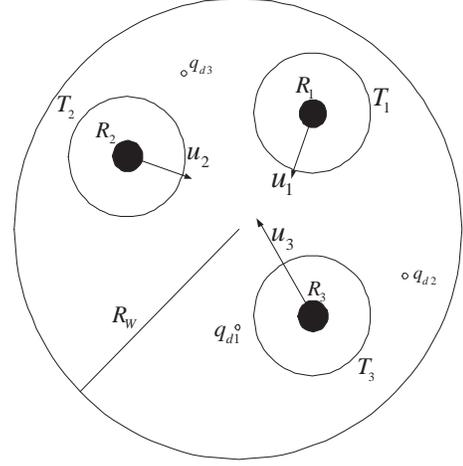
Fig. 1. A conflict scenario with three agents. Each agent  $i$  occupies a disc  $R_i$  (black discs) of radius  $r$  centered at  $q_i$ . The agents evolve in a bounded workspace of radius  $R_W$ . Each agent's sensing zone  $T_i$  (white discs) is centered at  $q_i$  and has radius  $d$ .
