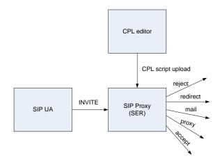
Figure 2: Call processing logic
