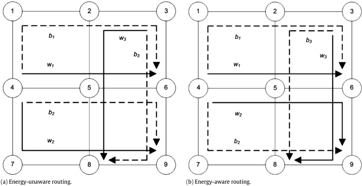
**Fig. 1.** Comparison of an energy-unaware and an energy-aware routing approaches.
