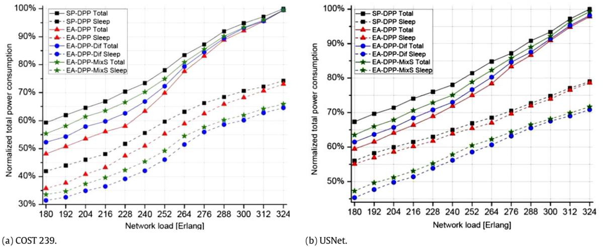
Fig. 3. Normalized total power consumption vs. network load for (a) COST 239 and (b) USNet network topologies.
