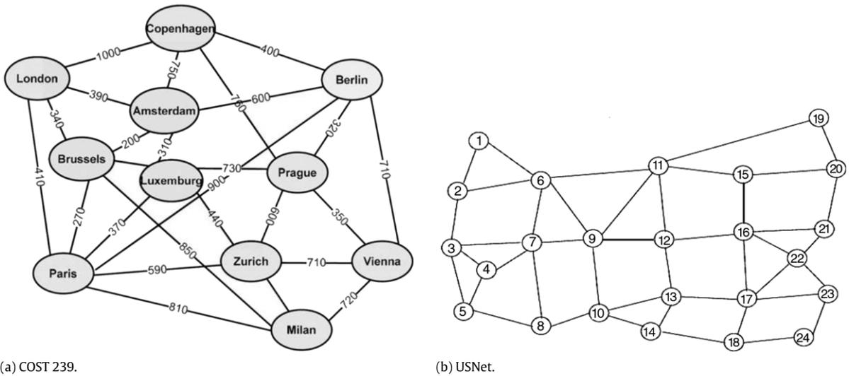
Fig. 2. (a) Pan-European COST 239 test network, and (b) sample US network USNet.
