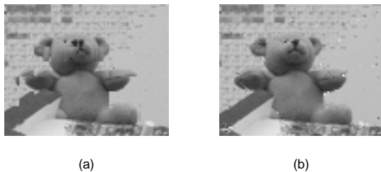
Fig. 8. Upper right quadrants of reconstructed images for Teddy showing (a) blocking artifacts using the decoder in [2] and (b) showing removal of block artifacts using the improved decoder. The side information image is Y_1 . Rate = 3.87 bpp.
