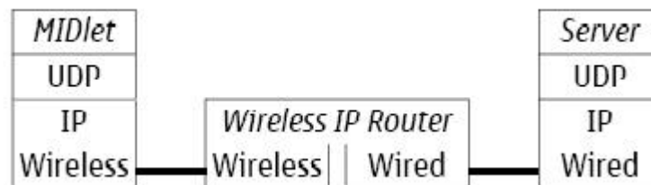
Figure 2-8: Structure of UDP over wireless network
