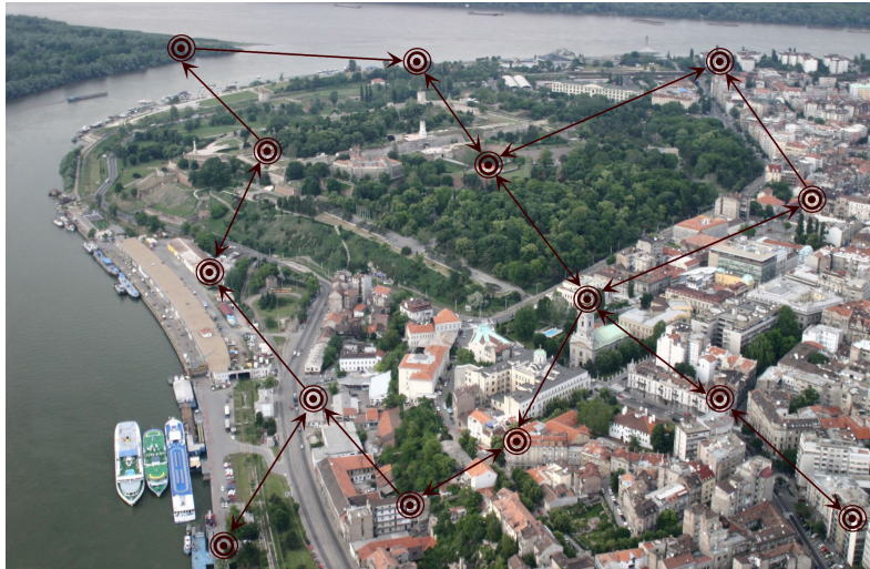
Figure 1. An example sensor network used in smart-city applications with decentralized communication topology. The inter-node communication is performed according to the depicted directed graph. The introduced distributed calibration algorithm achieves asymptotic calibration of all the sensor nodes in the network without using any type of fusion center.
