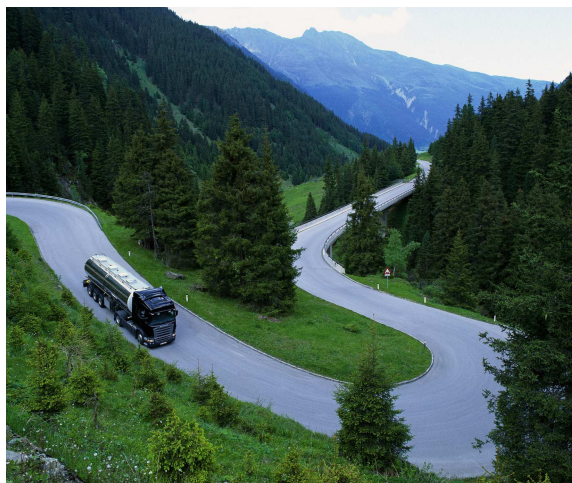
Fig. 1. When driving over a hill a preview information enabled cruise control could automatically lower the speed before the peak. Due to the many sharp bends in the road, braking will probably be inevitable at some point, and the auxiliary systems can be controlled to engage only when there is an energy surplus.
