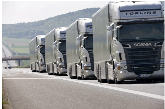
Fig. 1. Four heavy-duty vehicles platooning to reduce the fuel consumption for the following vehicles.
