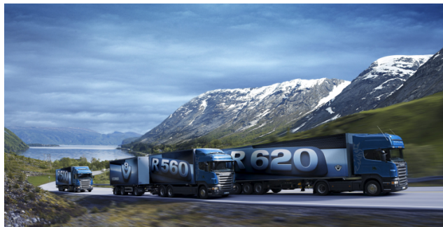
Fig. 1. Heavy duty vehicles traveling in a platoon can achieve significant fuel reduction.
