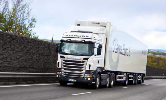
Fig. 13. A tractor-semitrailer vehicle with a 480 hp engine and 6 \times 2 configuration.
