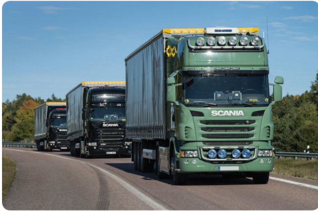
FIGURE 1 A platoon of three automatically controlled heavy-duty vehicles. The overall air drag is reduced as a result of small intervehicular distances, carefully regulated through vehicle-to-vehicle communication. (Image courtesy of Scania CV AB.)
