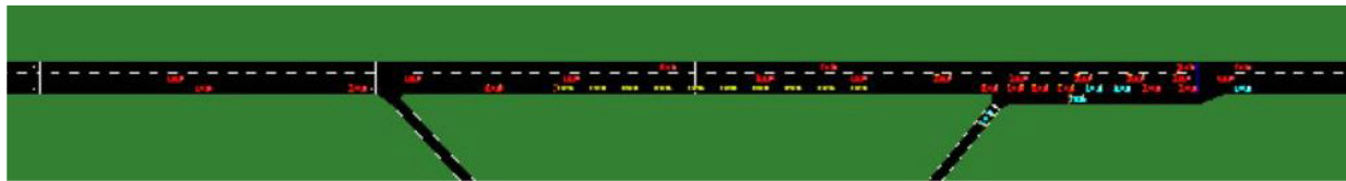
Fig. 11. Microsimulation environment. Red, cyan, and yellow vehicles represent mainline traffic, on-ramp/off-ramp traffic, and CAV platoons, respectively.
