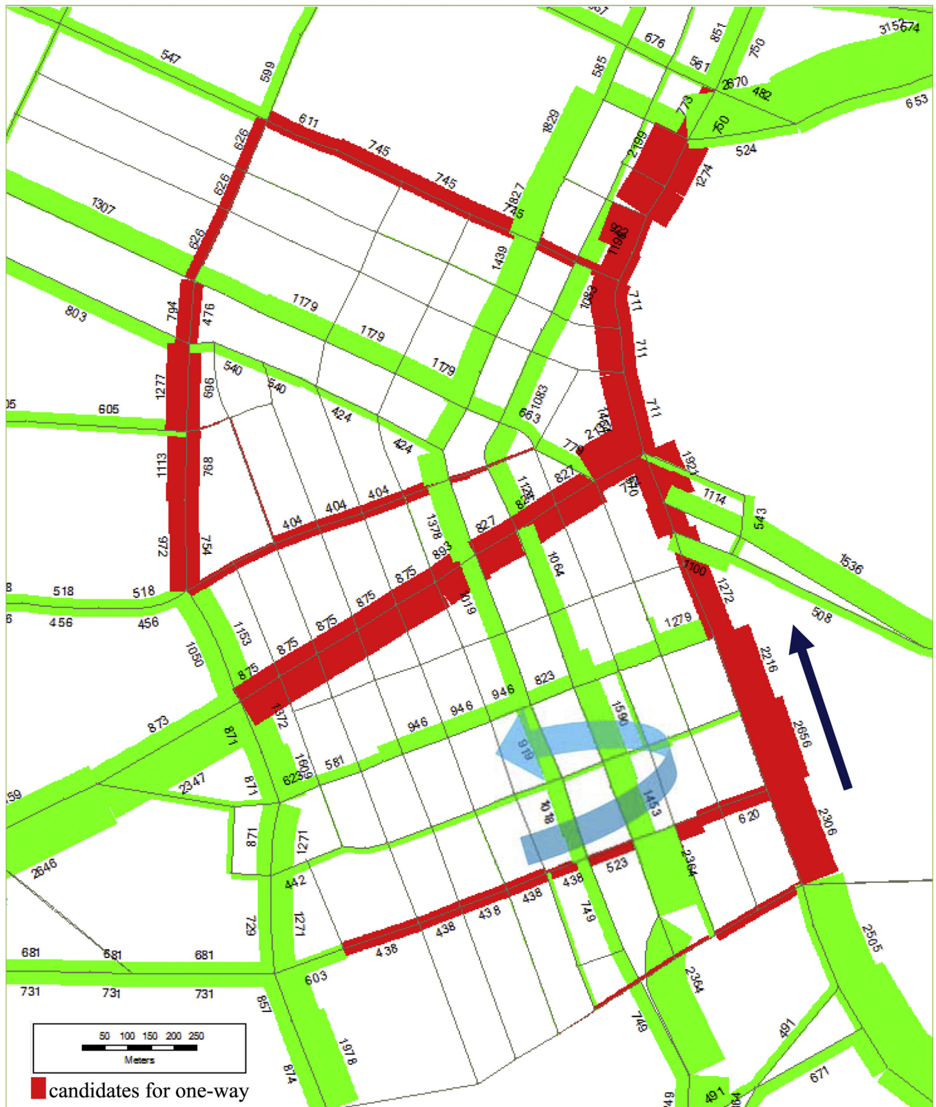
Fig. 4. Winnipeg case study, the CBD, traffic flow of the best contraflow (one-way) scenarios (the thickness of the roads indicates the relative size of their respective traffic volumes, the numbers indicate the traffic volumes in hourly rate).
