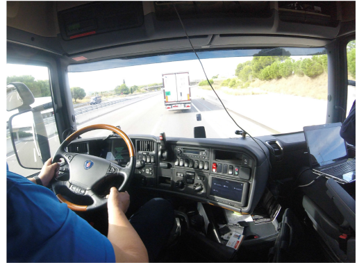
Fig. 13. View from the cockpit of the green vehicle while trailing the blue vehicle in the platoon. The on-board HMI can be seen in the dashboard. The computer on right side of the image is used to monitor and collect data from the on-board system.
