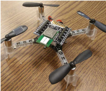
Fig. 10. CrazyFlie 2.0 quadrotor helicopter with UWB expansion.
