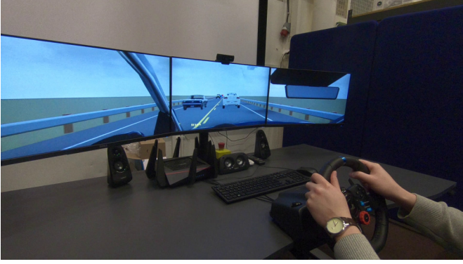
Fig. 8. The experimental setup for the overtaking scenario. illustrated in Fig. 6b with 3
