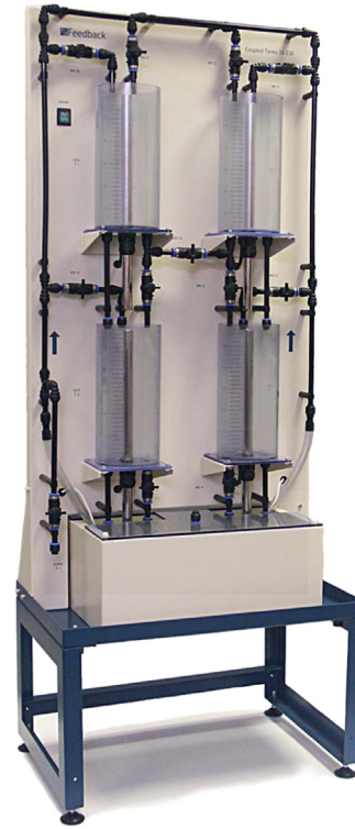
Fig. 2. Plant of four-coupled tanks.
