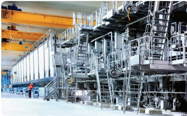
**FIGURE 3** Iggesund's paper mill has two paper machines that are 300 m long and produce state-of-the-art cardboard. The photo is taken from the wet end of the cardboard machine 2. At the far right of the photo is the wire section, where the pulp comes out of the headboxes and is dewatered on the wire. At that point, the pulp contains more than 99% water. To the left is the drying unit, where the cardboard is dried by steam. (Source: Iggesund Paperboard; used with permission.)
