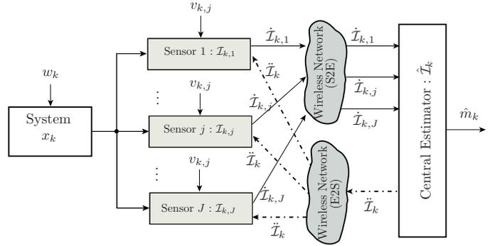
Fig. 1. Distributed event-triggered estimation system architecture.
