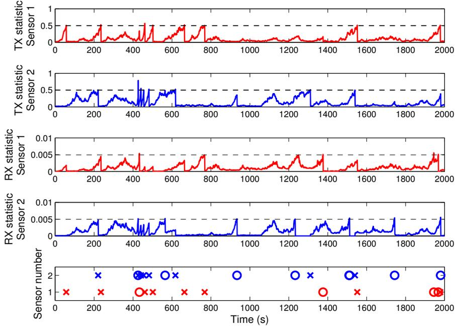
Fig. 3. Transmission and reception statistics for wireless sensor 1 and 2 in transient conditions; Transmissions is characterized by a cross ( $\times$ ) and receptions by a circle ( $\circ$ ). Tank 1 and tank 2 levels are shifted at time  $t = 400$  s and at  $t = 420$  s, sensor 1 avoids transmission since it receives information from the central estimator. The listening benefit is observed also for sensor 2 at time  $t = 934$  s and  $t = 1980$  s and for sensor 1 again at  $t = 1374$  s.
