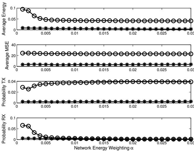
Fig. 5. Steady-state condition statistics in terms of average energy, MSE and probability of transmissions (TX) and reception (RX) for the case of: No tank level shift (Star (★)) and with periodic tank level shifting every 100 s (Circle (○)).
