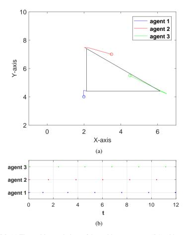
Figure 5.3: (a) The position evolutions of the multi-agent system (5.1) with event-triggered control input (5.4) when performing Algorithm 5.2. (b) The triggering times for each agent.
