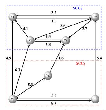
Figure 2.1: An example of a digraph which contains directed spanning trees. The subgraph in the dashed lines is the first strongly connected component, and the subgraph in the dotted lines is the second strongly connected component
