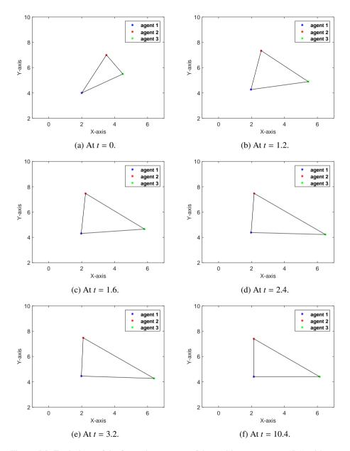
Figure 5.2: Evolutions of the formation process of the multi-agent system (5.1) with event-triggered control input (5.4) when performing Algorithm 5.2.
