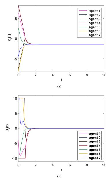
Figure 4.1: (a) The state evolutions of the multi-agent system (4.1)–(4.2). (b) The saturated input of each agent.
