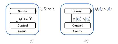
Figure 1.8: Illustration of how one agent gather information. (a) The case that the control input has the form (1.13). (b) The case that the control input has the form (1.14).
