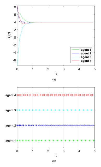
Figure 3.6: (a) The state evolutions of the multi-agent system (3.1)–(3.2) when performing Algorithm 3.1. (b) The triggering times for each agent.
