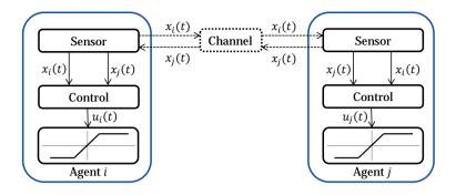
Figure 1.9: Illustration of how one agent communicates with another agent when the control input has the form (1.4). And the control signal is saturated before it is transmitted to the actuator.
