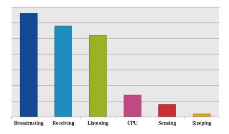
Figure 1.5: Typical power consumption of a wireless sensor [14].
