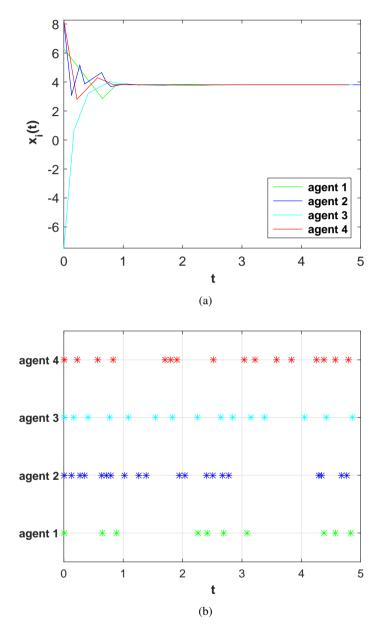
Figure 3.3: (a) The state evolutions of the multi-agent system (3.1)–(3.2) under the dynamic triggering law (3.11). (b) The triggering times for each agent.
