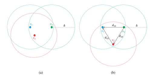
Figure 5.1: (a) The initial positions of three agents. (b) The desired formation  $\{d_{12}, d_{13}, d_{23}\}$ .
