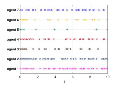
Figure 4.3: The triggering times for each agent in the multi-agent system (4.4)–(4.5) under the triggering law (4.6).
