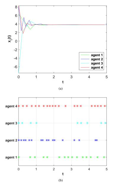
Figure 3.5: (a) The state evolutions of the multi-agent system (3.1)–(3.2) under the dynamic triggering law (3.27). (b) The triggering times for each agent.
