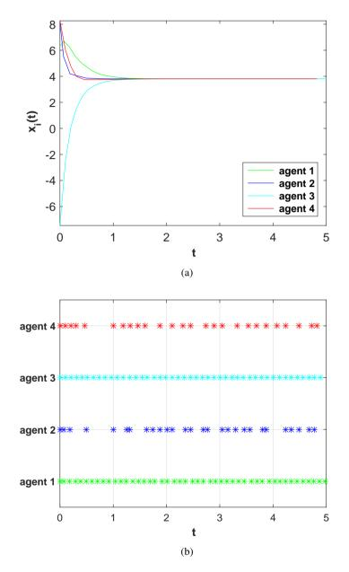
Figure 3.4: (a) The state evolutions of the multi-agent system (3.1)–(3.2) under the static triggering law (3.22). (b) The triggering times for each agent.
