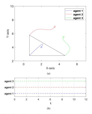
Figure 5.5: (a) The position evolutions of the multi-agent system (5.40) with event-triggered control input (5.46) when performing Algorithm 5.5. (b) The triggering times for each agent.
