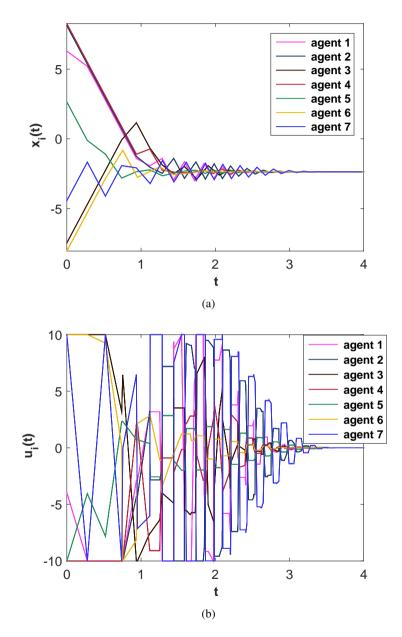
Figure 4.4: (a) The state evolutions of the multi-agent system (4.4)–(4.5) when each agent performs Algorithm 4.1. (b) The saturated input of each agent.
