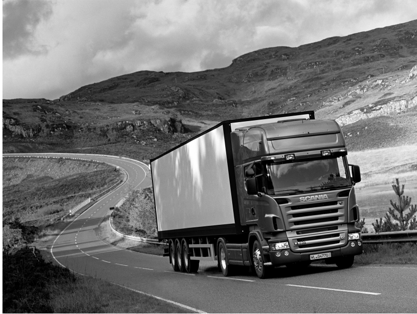
Figure 1.1: Scania R 580 4x2 tractor with a three axle semitrailer driving a country road in Great Britain.
