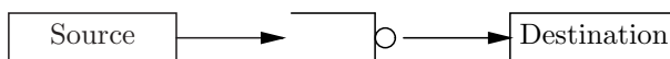
Figure 6.11: The simplest possible topology. A single data flow, with a single intermediate bottleneck router.
