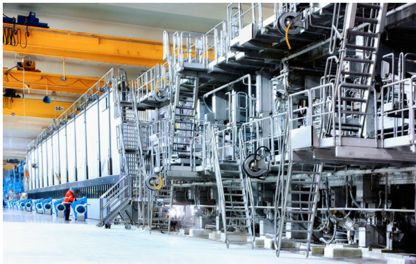
Figure 1.2: Paperboard machine in the Iggesund paper mill. High quality paperboard is manufactured in the machine after starch is mixed to coat the paperboard.
