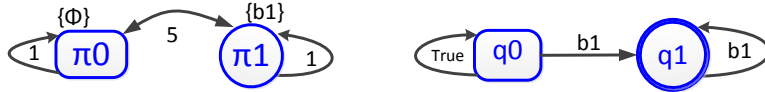
Figure 4.3: Agent 2's model and task: its FTS \mathcal{T}_2 (left) and NBA \mathcal{A}_{\varphi_2} associated with \varphi_2 = \Diamond \Box b_1 (right).
