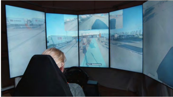
Figure 1.6: Teleoperation of trucks by Einride where human operators are able to control multiple autonomous trucks from a single remote drive station [20].
