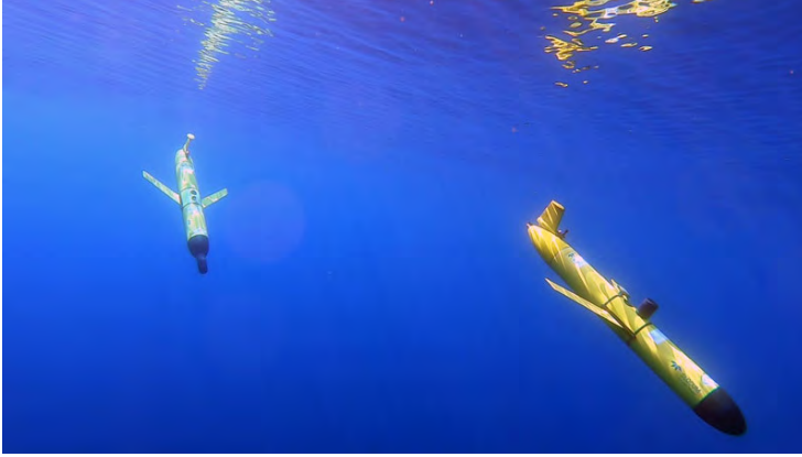
Figure 1.2: Autonomous underwater vehicles map the seafloor and analyze water properties. Source: https://transmitter.ieee.org/aUvs-how-autonomous-underwater-vehicles-protect-oceans-and-divers/
