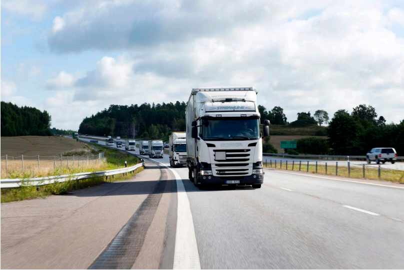
Figure 1.3: Heavy-duty vehicles can form platoons to reduce the air drag coefficient and thereby improve their fuel efficiency. Picture provided courtesy of Scania http://www.scania.com/ .
