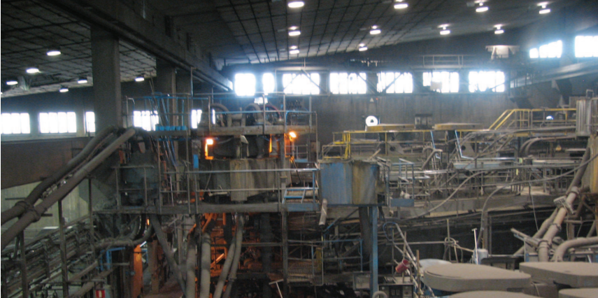
Figure 1.1: An IEEE 802.15.4-based wireless control of the froth flotation process at Boliden was tested within the SOCRADES EU project ( http://www.socrades.eu/ ).
