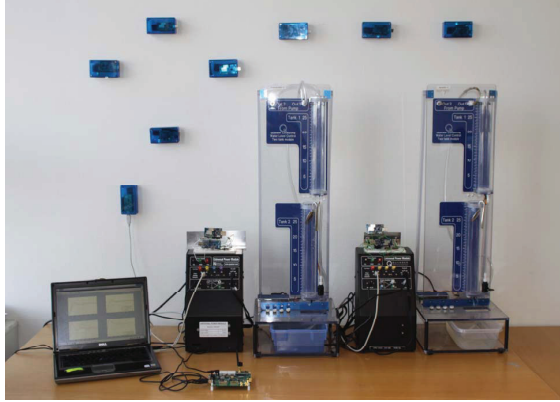
Figure 4.1: Lab process with a wireless network. Two double-tank systems share the wireless network with eight wireless nodes performing monitoring tasks.
