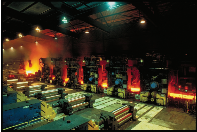
Figure 1.1: A hot rolling mill composed of a sequence of rolling stands yielding the desired steel bar section as the bar moves through the mill. (Courtesy of ABB)
