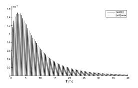
Fig. 4. Condition (13) is depicted in the this case for agent 3. The solid line shows the evolution of  $|e_3(t)|$ . This stays below the specified state-dependent threshold given by (13)  $|e_3|_{\max} = \sqrt{\frac{\sigma_3 a(1-a|N_3|)}{|N_3|}} z_3$  which is represented by the dotted line.
