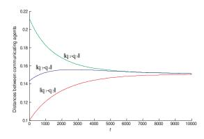
Fig. 1. Four single integrator agents are driven by the control (4) with  $\gamma$  as in (6). The formation graph is a tree. Agents' relative distances are stabilized to the expected desired value d=0.15.
